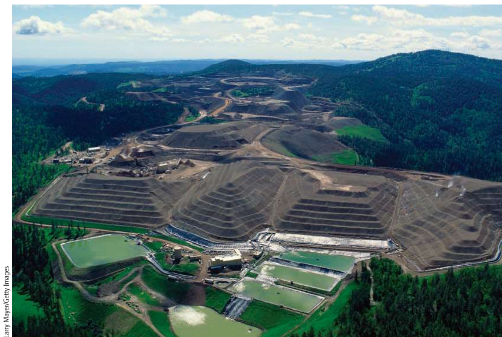
FIGURE 14.1 Gold mine in the Black Hills of the U.S. state of South Dakota with cyanide leach piles and settling ponds in foreground.
