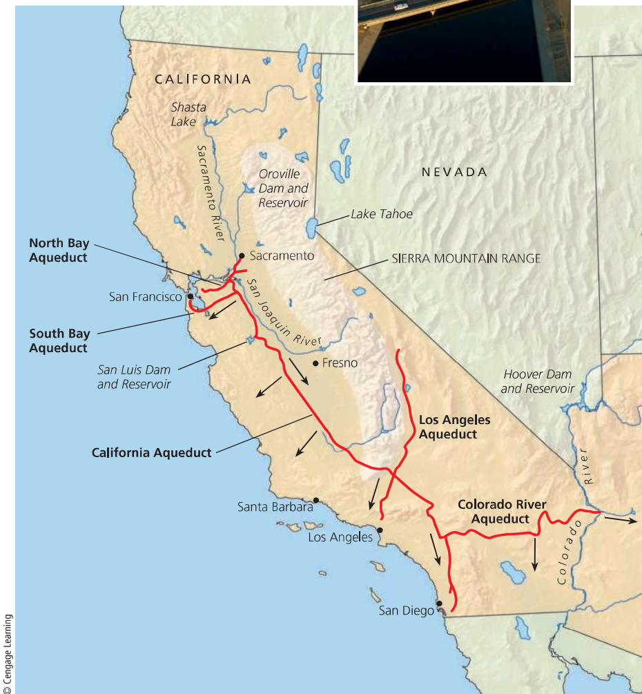
FIGURE 13.17 The California State Water Project transfers huge volumes of freshwater from one watershed to another. The arrows on the map show the general direction of water flow. The photo shows one of the aqueducts carrying water within the system. Critical thinking: What effects might this system have on the areas from which the water is taken?
