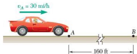
$$11.35) a = 11 \text{ ft/s}^2 \quad \text{in A; } (x=0, v=30 \text{ mi/h}) \quad 30 \text{ mi/h} = 44 \text{ ft/s}$$
