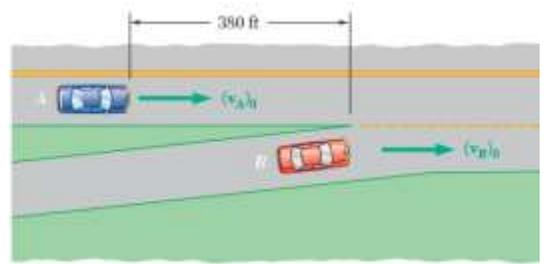
11.75) Para B:  $60 \text{ mi/h} = 88 \text{ ft/s}$      $15 \text{ mi/h} = 22 \text{ ft/s}$
